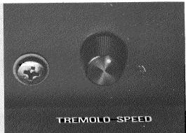
The Electone's special throbbing tremolo is produced by a smaller-size Natural Sound speaker that actually spins just behind the tremolo speaker grille on the side of the cabinet.
