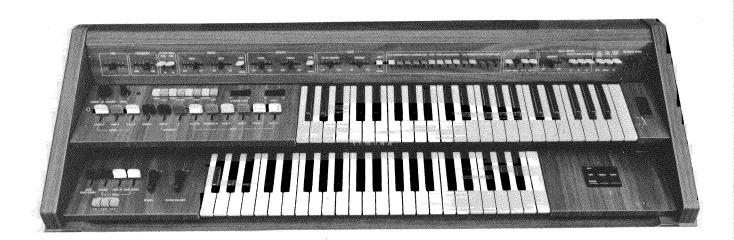
Your CSY-1 has 14 preset tone levers on the front panel . When you depress one of the levers and push a note, you hear the sound of the instrument voice identified by name on the lever panel. It is designed to create the sound of
