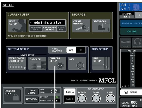
Pulsante OUTPUT SETUP (CONFIGURAZIONE PORTA DI USCITA)
