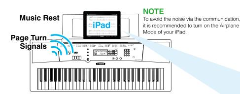
Playback of the Preset Song outputs a special sound signal (referred to as "Page Turn Signals") for turning the score page as playback progresses. The Page Turn Signals that is input to the iPad microphone calls up the corresponding score on the screen.
