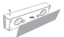
**4-2** With the help of another person, hold the Speaker unit horizontally, and slide it from the rear into place along the brackets.
