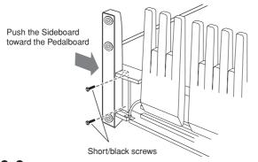
**3-3** Stand the Pedalboard after securing the screws.
