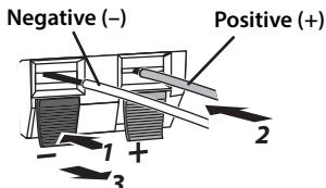
**Note:** Make sure the terminal is gripping the bare wire, not the insulation.
